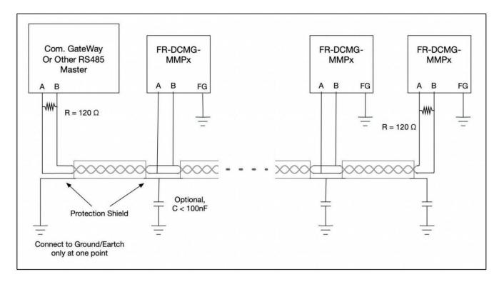
The wiring of on-site communication lines requires that the communication shield can only be grounded at a single point, otherwise there will be a risk of lightning surge damage to all equipment on the entire communication line during a lightning strike; If you encounter a situation where communication line
