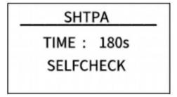
On the shunt trip setting interface, you can set the shunt trip enable time (TIME) and trip self-check (SELFCHECK) when an arc alarm occurs.
