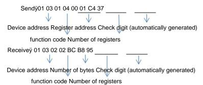
Message example analysis: The above sending message reads the value of slave address 1 and register address 0x0104 (voltage V), and the received message responds with voltage data 0x02BC, which is converted to decimal, which is 700V.
